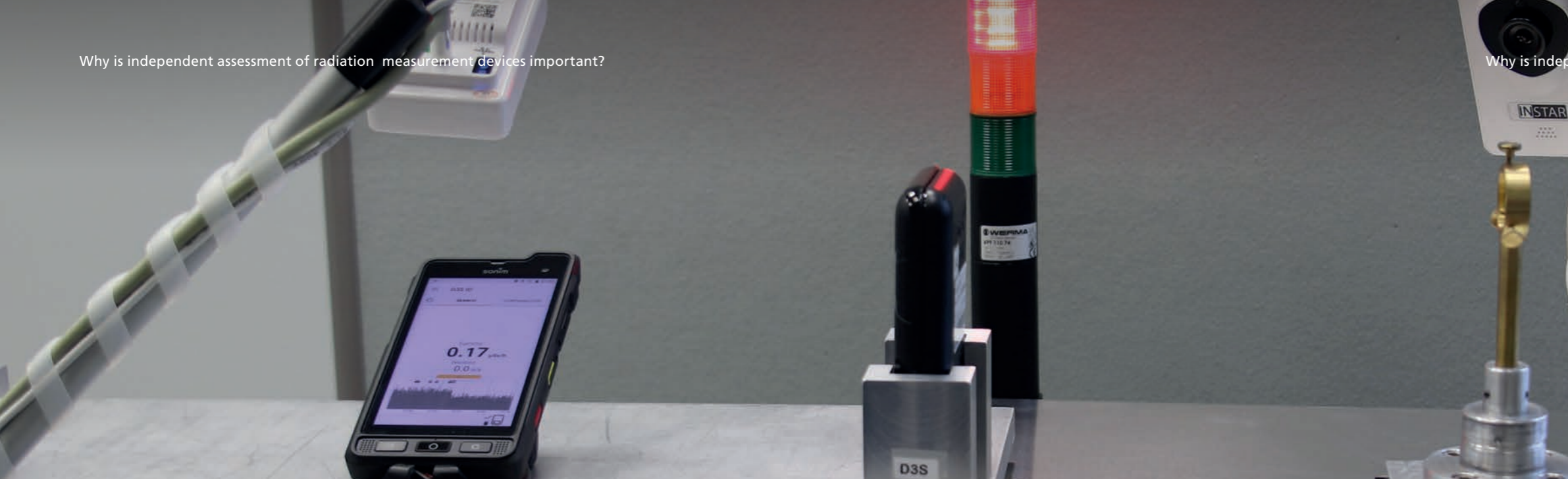
Measurement setup with D3S in front of radioactive source in the source lifting mechanism of the QuTeSt (smartphone used as display unit and detector in front of alert light).
