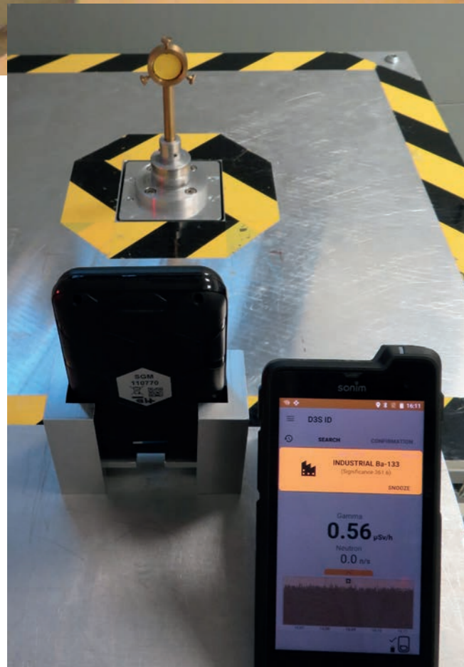
D3S in front of radioactive source (yellow) in the source holder of the source lifting mechanism of the QuTeSt.
