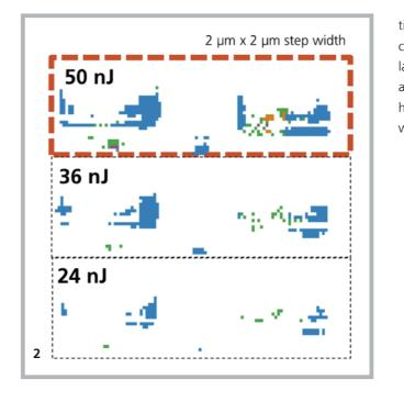
In Figure 2, the white dotted section roughly outlines one of the data channels of the Digital Isolator 14850 (step width in x and y direction 5  $\mu$ m). Figure 3 shows the red outlined area in finer resolution, as dependent on laser intensity (step width 2  $\mu$ m).
