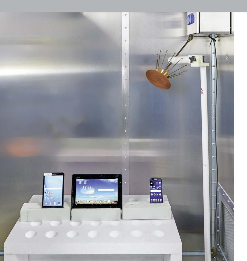
in the Gigahertz range, to reflect the growing number of applications in modern sensor and communications technology at such frequencies. Additionally available are a small anechoic chamber and a wide variety of high frequency and microwave measurement instruments.
