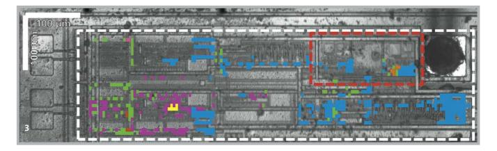
tified which under laser bombardment cause a latch-up on the component (blue). A possible explanation for the occurrence of latch-ups, which were not observed in previous heavy ion tests according to ESCC 25100 heavy ion tests, may be the known higher penetration depth of the 1064 beam in silicon, compared with the shorter range of the heavy ions used at the time.
