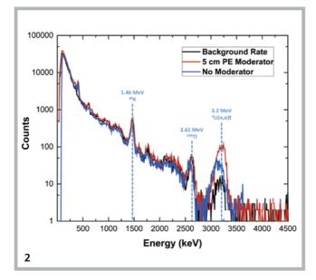
The investigation results on Li-6 based detectors at Fraunhofer INT show that materials with this isotope are very well suited for neutron detection, that the gamma detection which is simulta-
