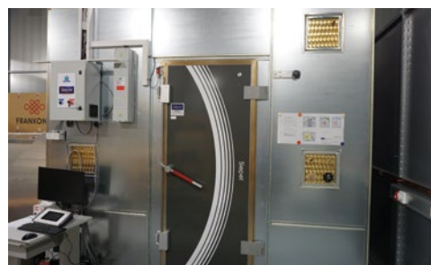
Fig. 2: New mode stirred reverberation chamber
